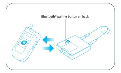
2. Under the list of available devices, select uDirect. Some phone models will Bond with uDirect. If you are prompted to Bond with uDirect, confirm with YES. When asked for the passcode or passkey, enter 0000 (four zeros). uDirect will be added to the Bluetooth devices list. Allow devices to complete the pairing process. On the cellular phone, uDirect is shown as a paired device and on uDirect, the Bluetooth LED indicator flashes slowly, indicating that the devices are successfully paired.
