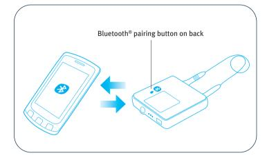
2. Under the list of available devices, select uDirect and enter 0000 (four zeros) when asked for the passcode or passkey. Allow devices to complete the pairing process. On the cellular phone, uDirect is shown as a paired device and on uDirect, the Bluetooth LED indicator flashes slowly, indicating that the devices are successfully paired.
