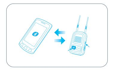
On the cellular phone, uDirect 2 is shown as a paired device and on uDirect 2, the Bluetooth LED indicator flashes slowly, indicating that the devices are successfully paired.
