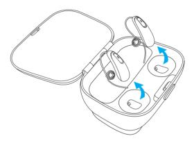
① Do not hold the tubes to remove the hearing aids from the charger as this can damage the tubes.
